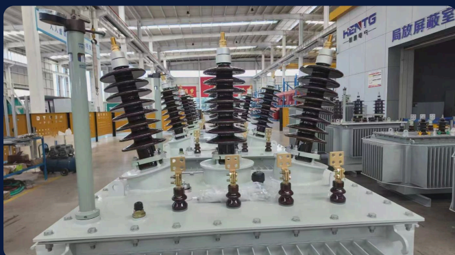
Oil-immersed transformers in final assembly at the factory.
