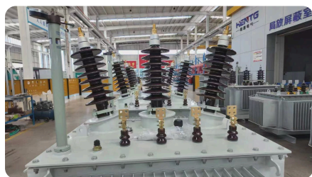
Transformers in final assembly at the factory.
